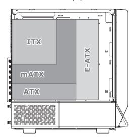
CPU cooler max height: 185mm
