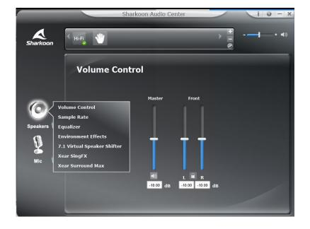
Through the Sharkoon Audio Center, control the volume of the speakers, make changes to the sound via the equalizer, access a variety of pre-installed effects, and configure the simulated position of the 7.1 surround sound. To access the individual menu items, right-click on the speaker symbol on the left side of the software.
