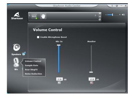
The Sharkoon Audio Center enables setting customization for audio recording via the microphone. To access the individual menu items, right-click on the microphone symbol displayed on the left side of the software.
