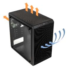
**Excellent thermal performance** The open design of the perforated front, top, and bottom guarantees excellent thermal performance.
