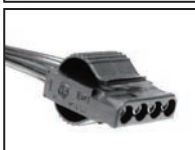
4Pin Peripheral Connector Head
