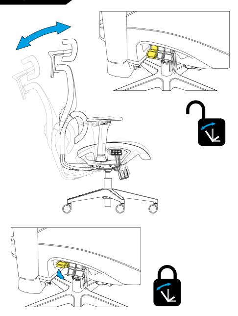
Once unlocked, slight pressure must first be applied to the backrest before the chair is released from the currently locked angle.
