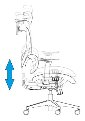
The chair can only be lowered when there is pressure on the seat base. The chair can only be raised when there is no pressure on the seat base.
